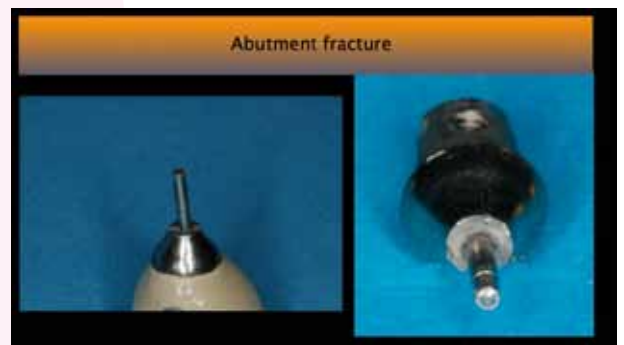
Figure 4b. Abutment fracture due to overload in terms of occlusal forces, abutment strength and design.
